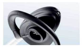
**Rocker switch and speaker** The rocker volume control is both intuitive and easy to use. Use it to adjust headset speaker volume during a call or to mute the outgoing signal.
